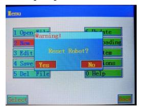
Left function key is yes, right function key is no; after selection, the system will automatically pop up the file saving dialog box, input the file name, and press save to enter the instruction teaching editing dialog box (the "#" key is the number and letter switch key. ) The instruction shown on this screen will be automatically saved in the file just entered. As shown in the figure :
